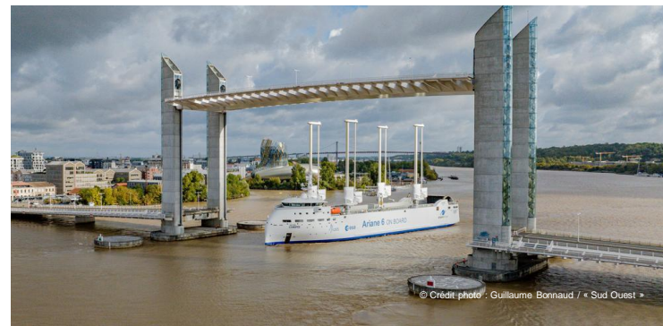
Canopée, 121 metres, hybrid wind-powered industrial cargo ship to transport Ariane 6 from Europe to Kourou
