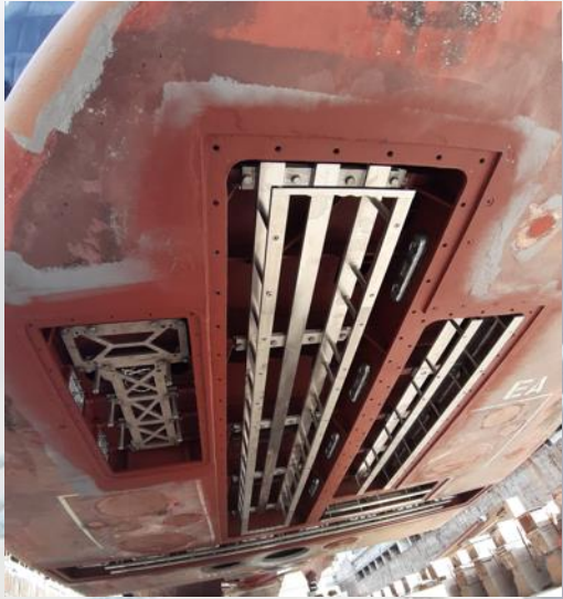
NEW FRAME INSTALLATION
