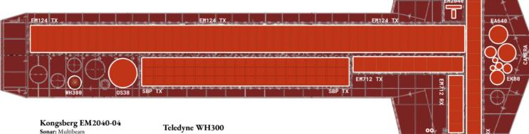
Degree: 0.25° x 0.5° Depth Range: < 1m - 635m Operating Frequency: 200 - 700 kHz Swath Width: Up to 170° Receiver Beams: 1024 beams
