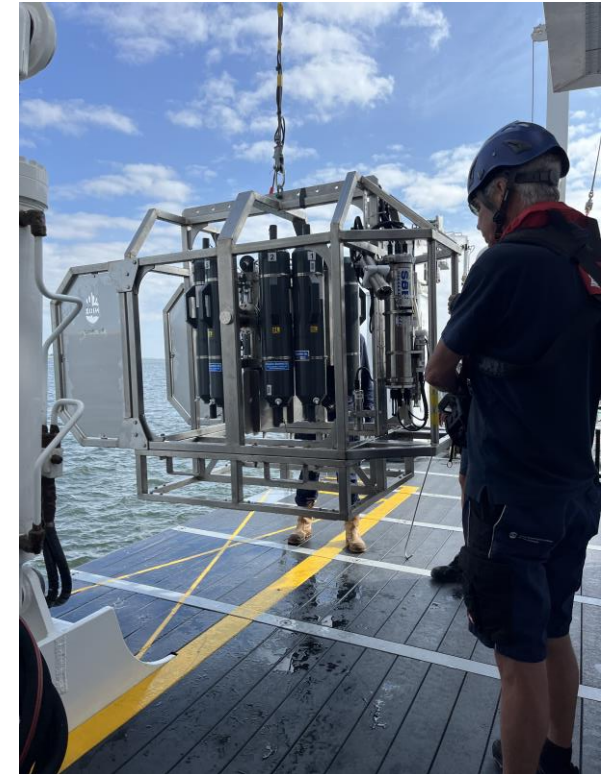
Custom-built CTD system for RV Wim Wolff
