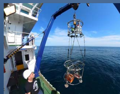
Lander deploy and recovery using the LanderPick system.
