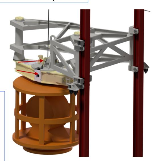
Special attention has been given to allow for launch and recovery for a wide variety of equipment while keeping setup/rigging time to a minimum. Scientific docking head on a-frame and moonpool cursors has been designed for moving equipment between A-frame and moonpool without requiring retermination of umbilical.
