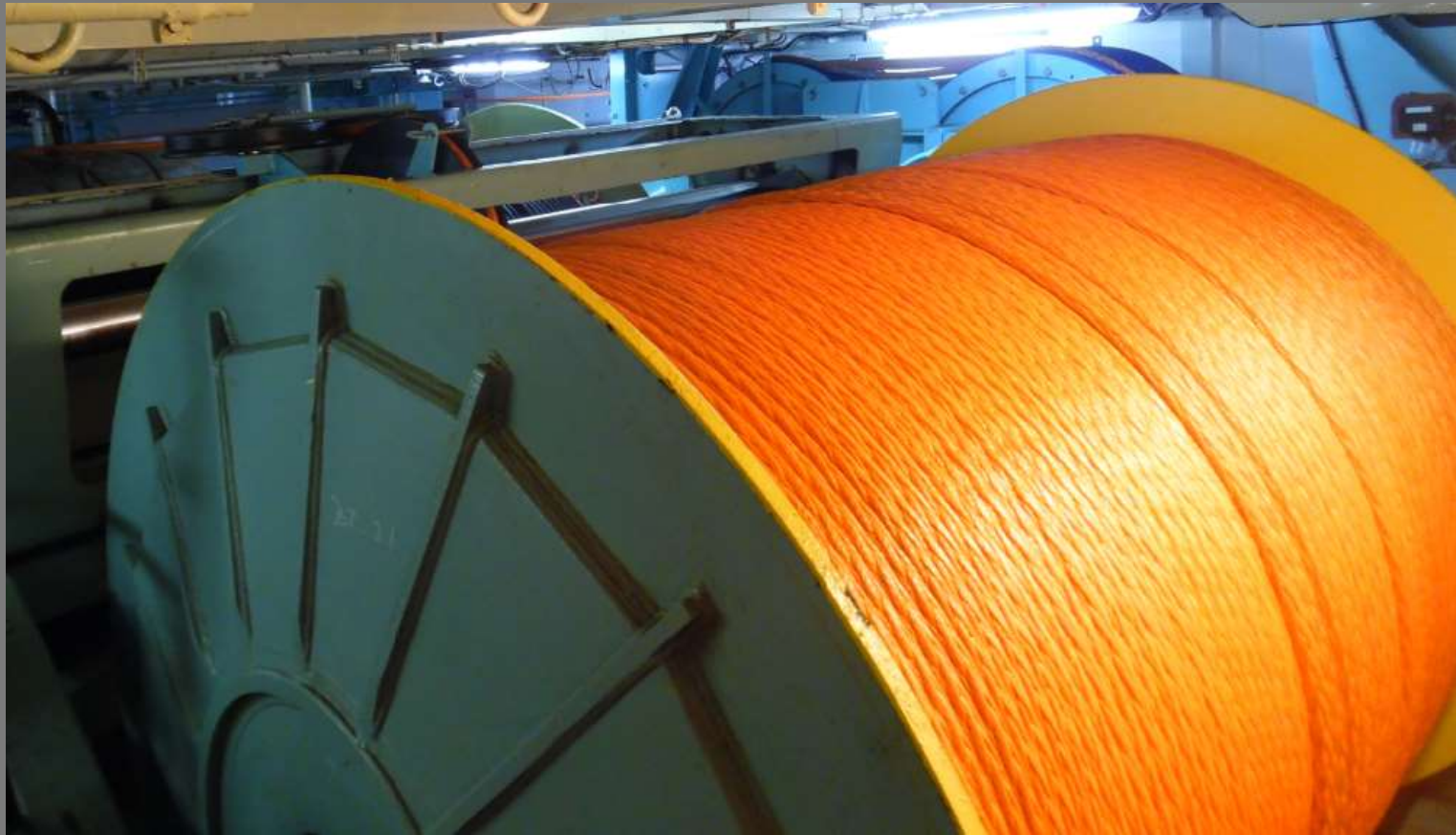
Special design of braiding of Dynalight cable \varnothing 35\text{mm} – as stiff as possible
