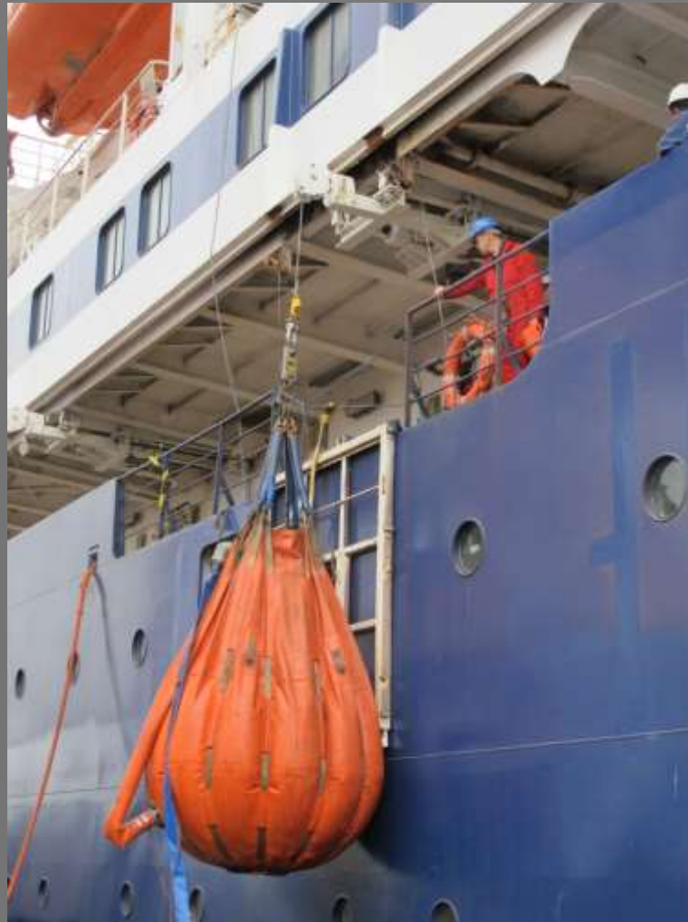
Load tests for telescopic booms for long core handling
