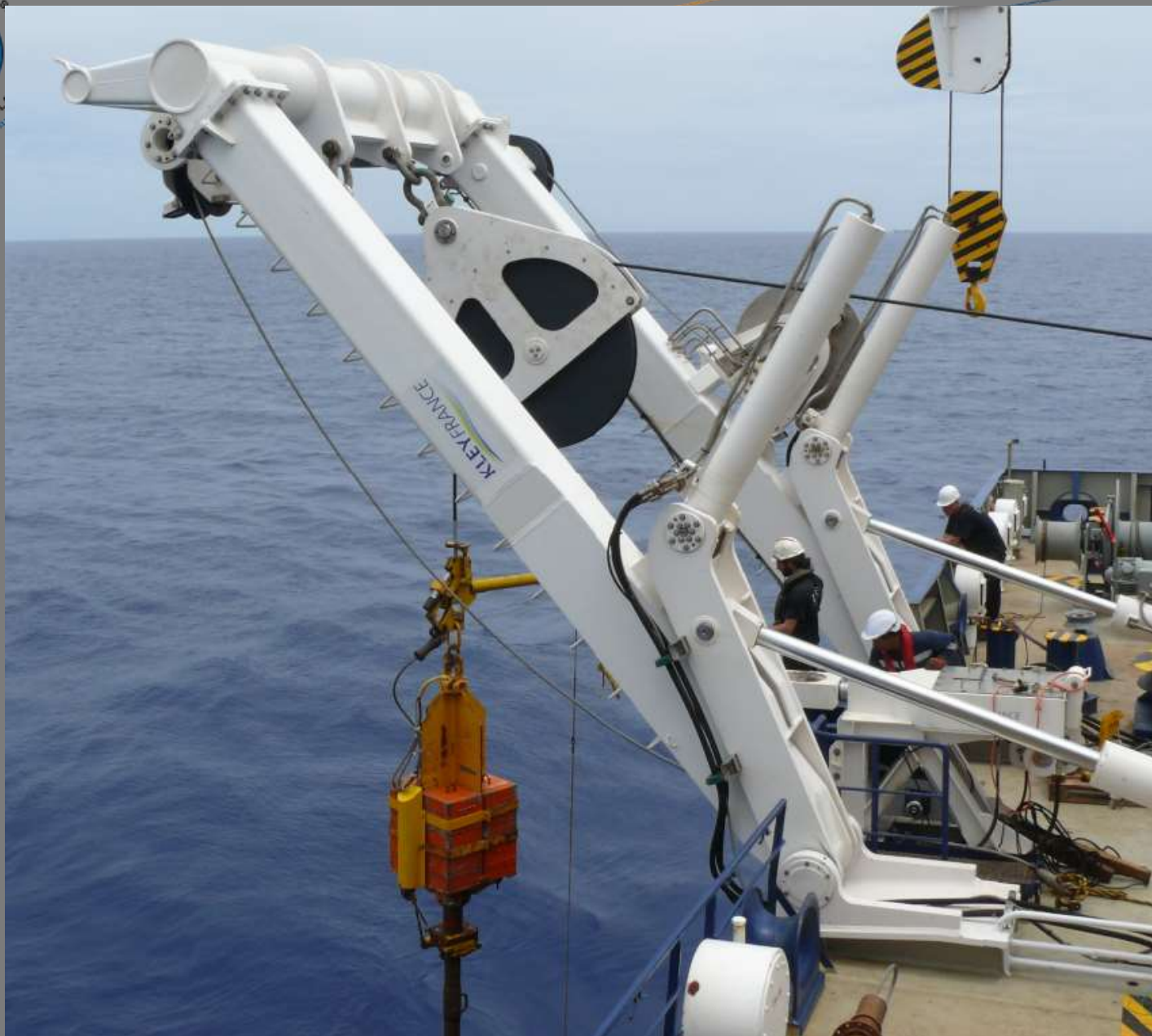
Coring A-frame : SWL 45T, top frame shifted, integrated handling winch
